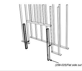
Secure horizontal steel header stud with 2 screws per side as per diagram.
