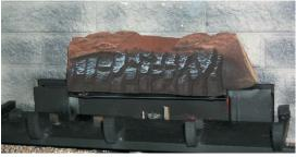
4) Place Log <u>02-51</u> on the front right side of the burner. Push the back of the log against the 2 brackets with the notch on the bottom right side of the log fitting into the right side of the grate.
