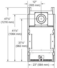
Framing dimensions in illustrations accommodate 1/2" finishing material.
