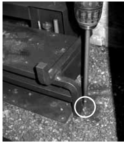
Diagram 1: Remove the left and right screws.
