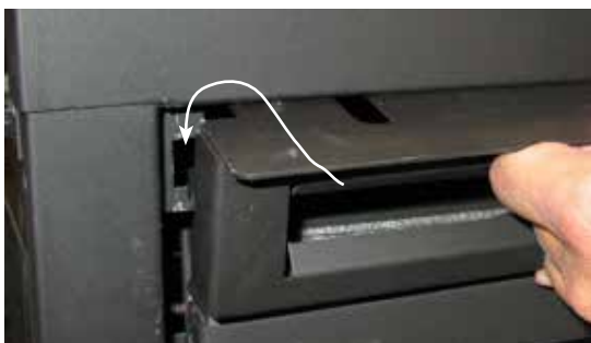
Installation of upper Flush Panel
